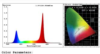
Chromaticity Coordinate:x=0.3354 y=0.2214/u'=0.2691 v'=0.3996 CCT=4553K(Duv=-0.0808) Dominant WL:Ld =-553.6nm Purity=33.4% Ratio:R=32.6% G=59.8% B=7.6% Peak WL:Lp=660.9nm FWHM=19.3nm Render Index:Ra=27.9 AvgR=21.0 R1 = 0R2 =37 R3 =81 R4 =16 R5 = 0R6 =38 R7 = 52R8 =0 R9 = 0R10=0 R11=5 R12=0 R13=3 R14=82 R15=0
